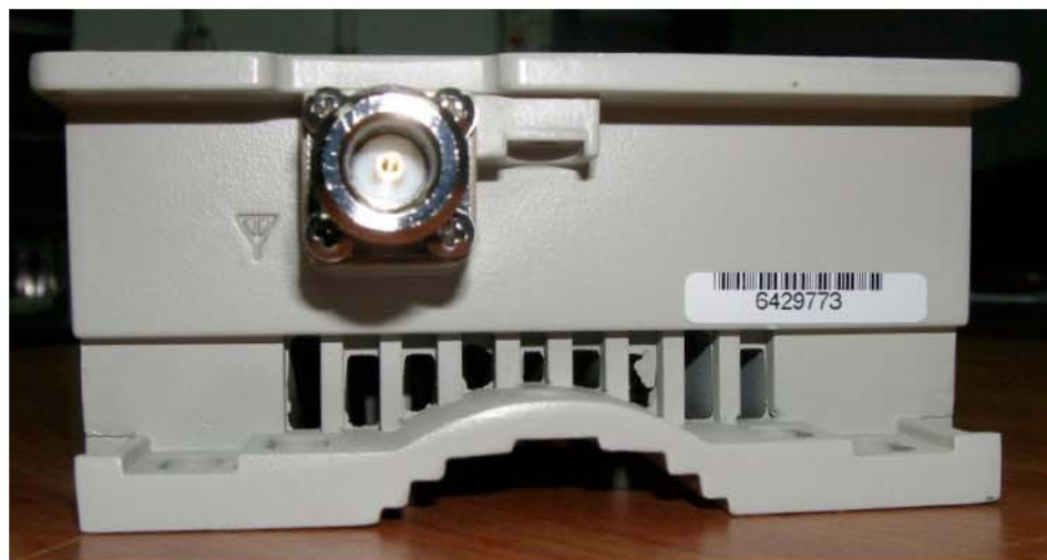
Photo # 4. Radio unit. RF & RJ45 connectors view
