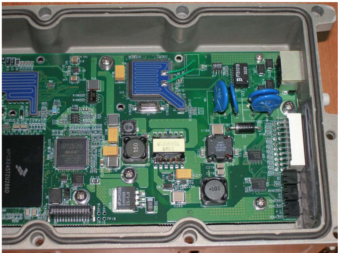
ODU components side , digital part
