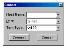
5. In the *Host Name* field, enter the IP address of the unit to be managed.
