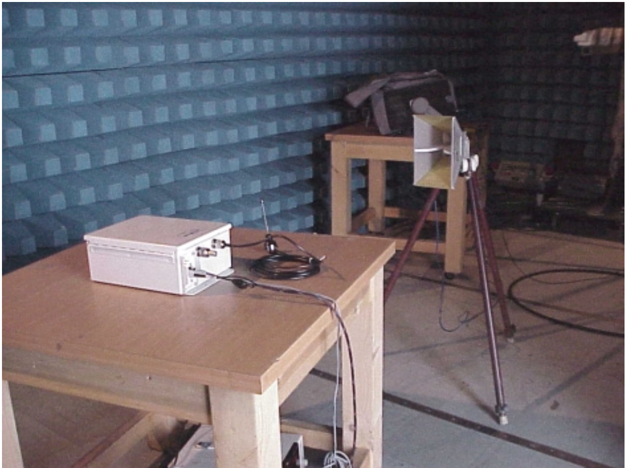
Photo 5. BreezeAccess SU-M unit Spurious emission test setup in semi -anechoic chamber
