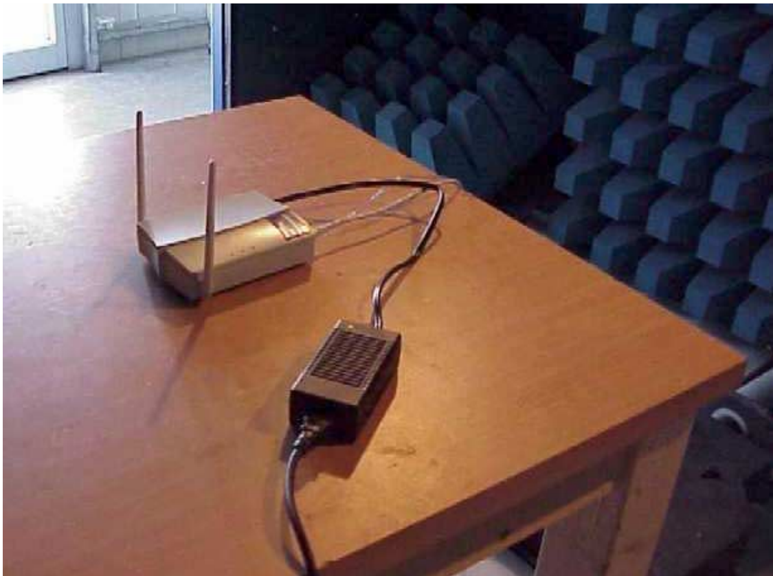
Photo #10 6dBi Omni antenna test configuration
