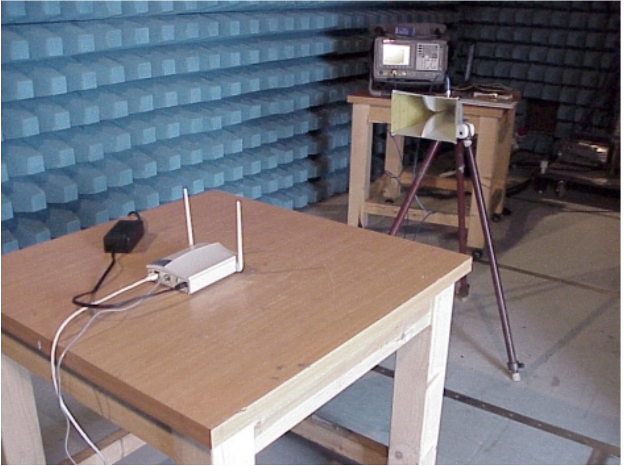
Photo #8 6dBi Omni antenna test configuration
