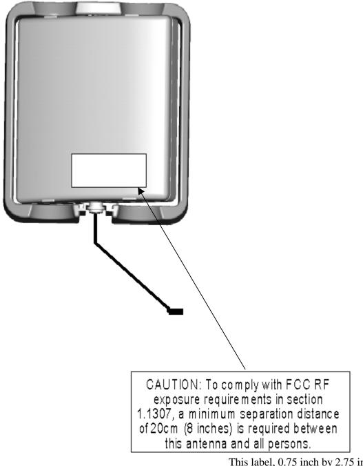
This label, 0.75 inch by 2.75 inch, 10pt black type, is placed on the front of the antenna.
