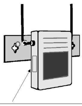
CAUTION: To comply with FCC RF exposure requirements in section 1.1307, a minimum separation distance of 20cm (8 inches) is required between this antenna and all persons.
