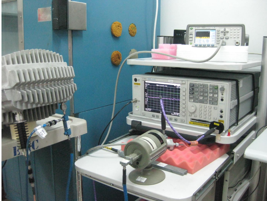
Photograph No.1 Conducted spurious emissions measurement setup
