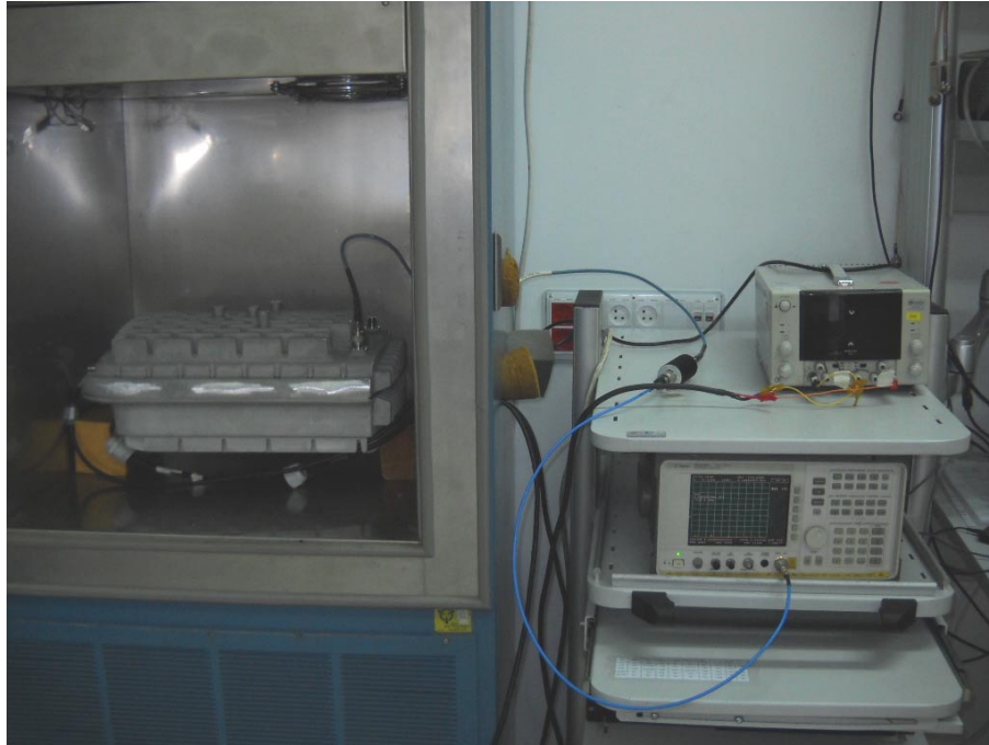
Photograph No.7 Frequency stability measurement setup
