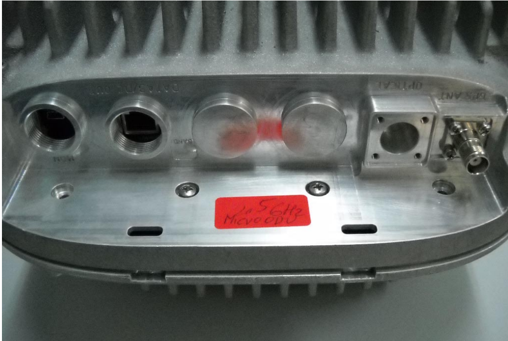
Photograph No.3 BreezeMAX Micro Outdoor microbase station connectors view
