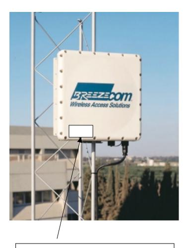
CAUTION: To comply with FCC RF exposure require ments in section 1.1307, a minimum separation distance of 56cm (22 inches) is required between this antenna and all persons.
