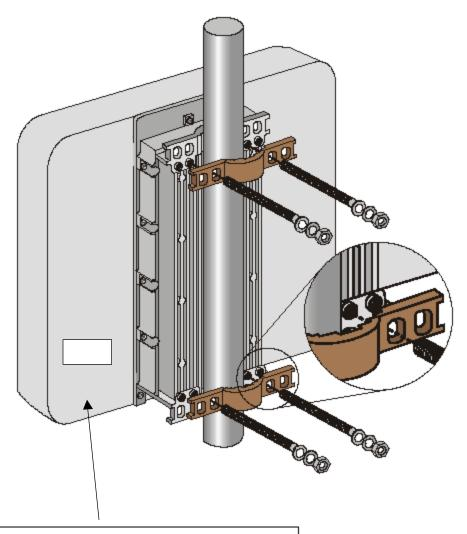
CAUTION: To comply with FCC RF exposure require ments in section 1.1307, a minimum separation distance of 56cm (22 inches) is required between this antenna and all persons.
