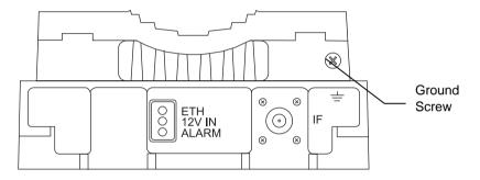
Figure 2-3. AU-RA/AU-RE Radio Unit Bottom Panel
