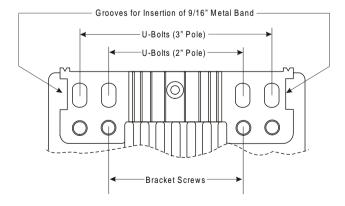
Figure 2-1. Holes/Grooves/Screw Holes
