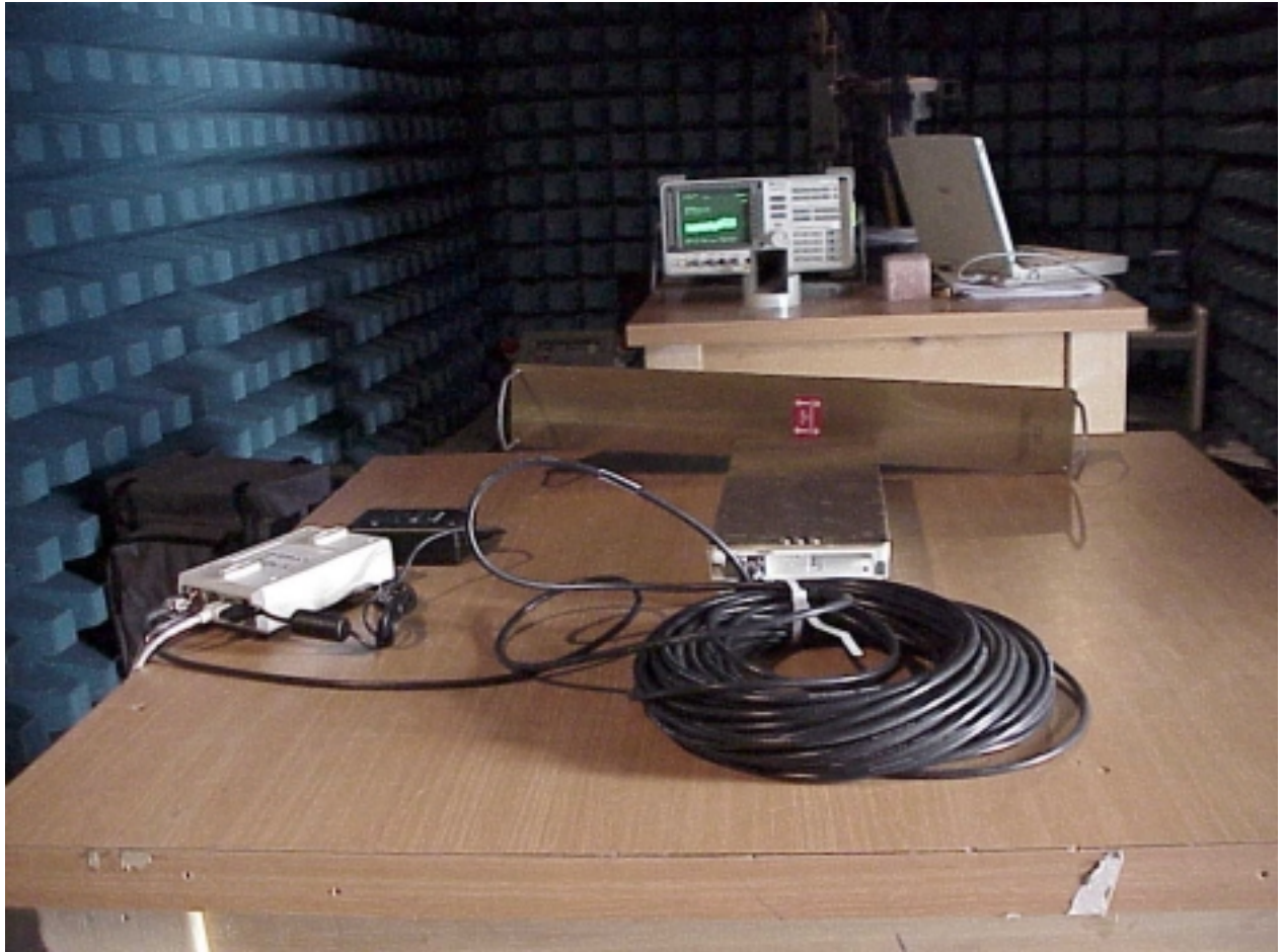
Photo #8 EUT with sector antenna. Radiated emission test
