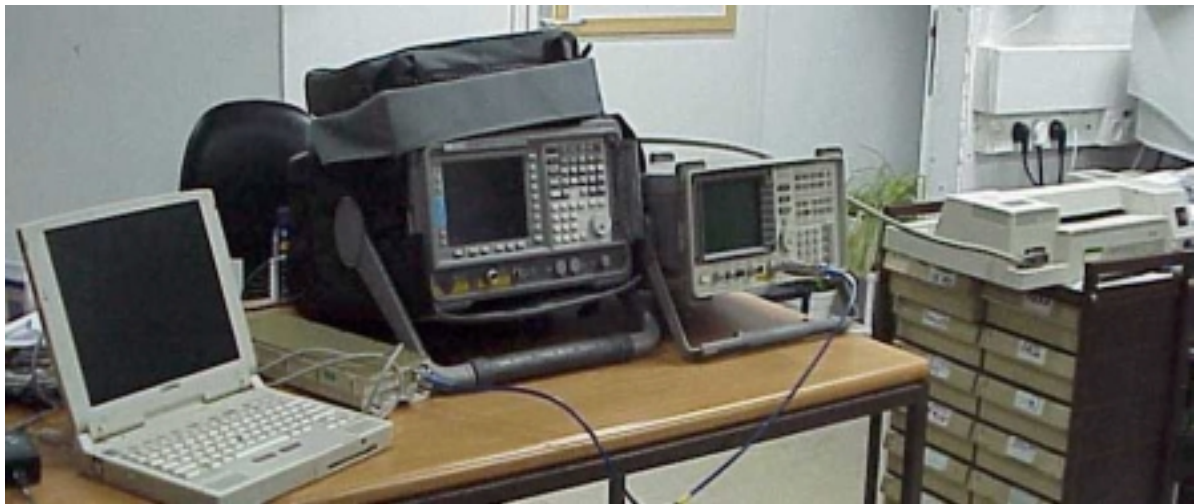
Photo #10 Spurious conducted antenna test. Measuring equipment
