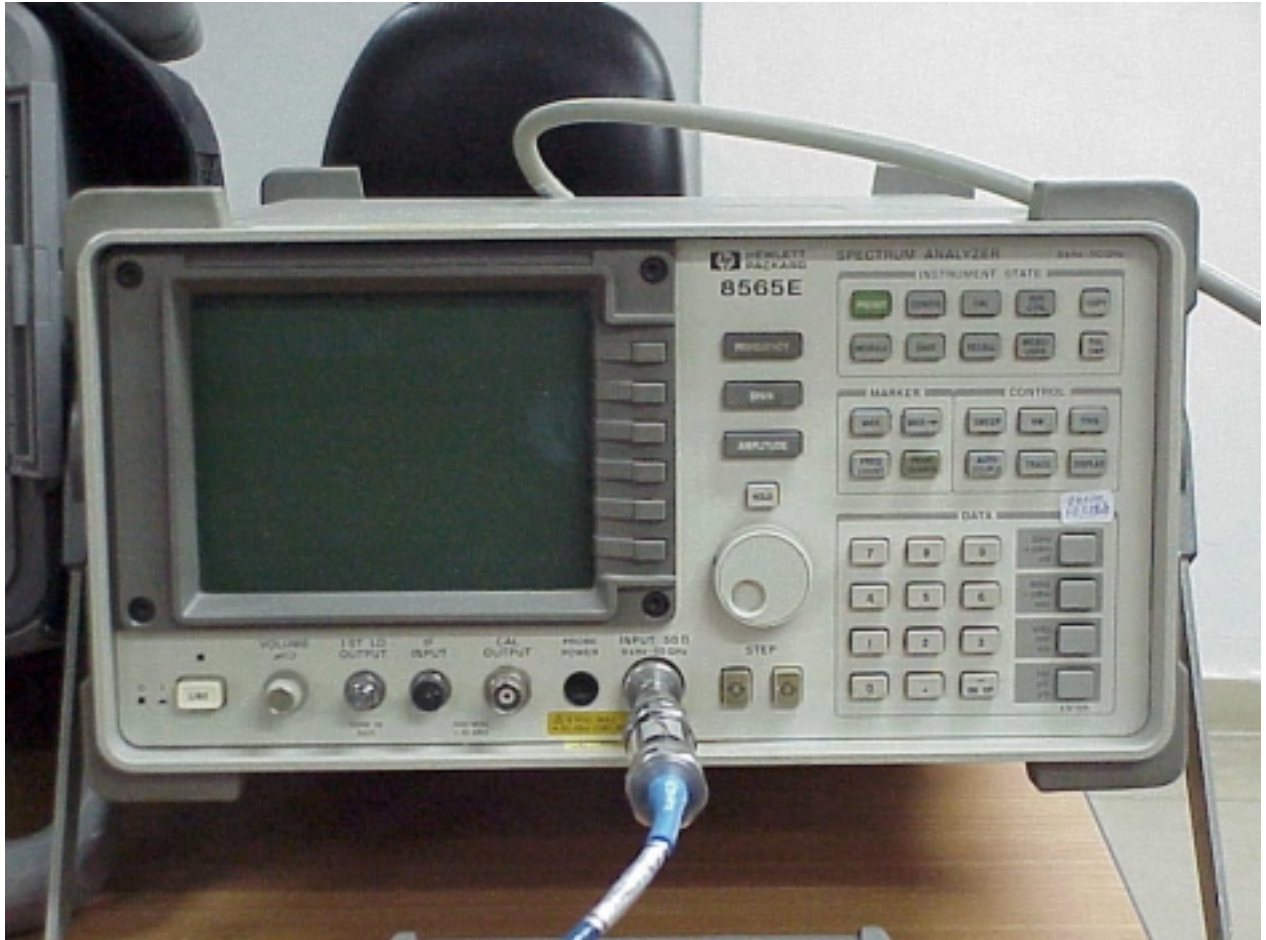
Photo #11 Spurious conducted antenna test. Measuring equipment
