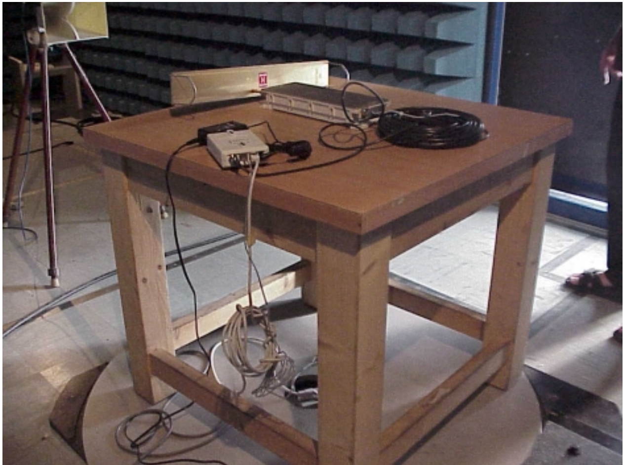
Photo #6 EUT with sector antenna. Radiated emission test
