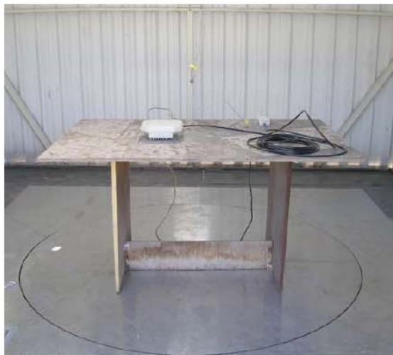
Photo #3. Radiated emissions test setup on OATS.
