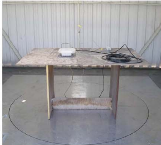
Photo #3. Radiated emissions test setup on OATS.
