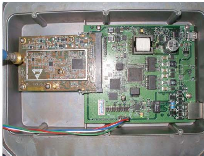
Photo #4. Outdoor unit. Internal view.
