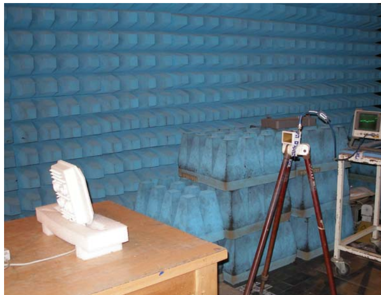
Photo #2. Radiated emissions test setup. Investigation test at 1m test distance.
