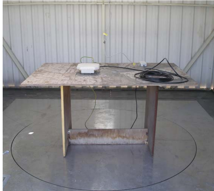
Photo 3. Radiated emissions test setup on OATS.
