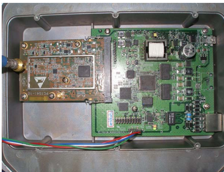
Photo 4. Outdoor unit. Internal view.
