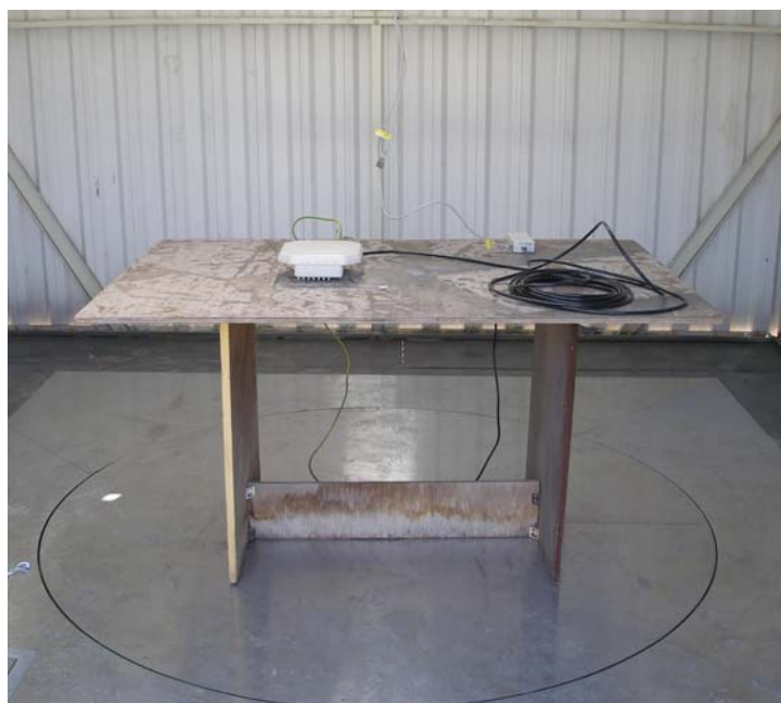
Photo 3. Radiated emissions test setup on OATS.
