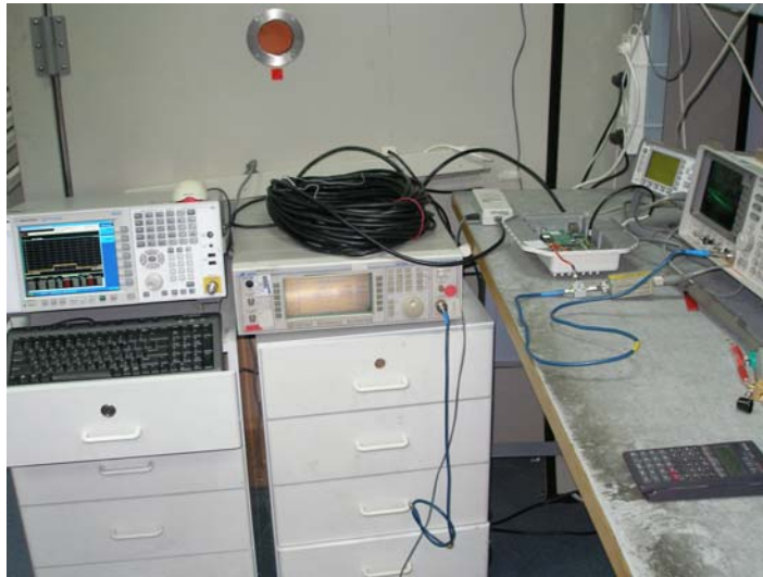
Photo #1. RF conducted emissions test setup.
