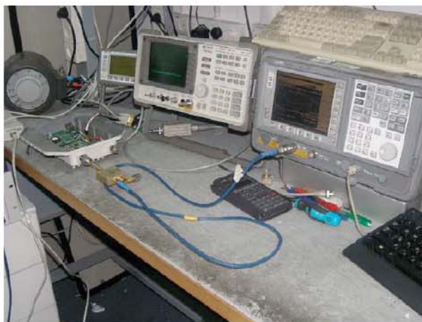
Photo #1. RF conducted emissions test setup.
