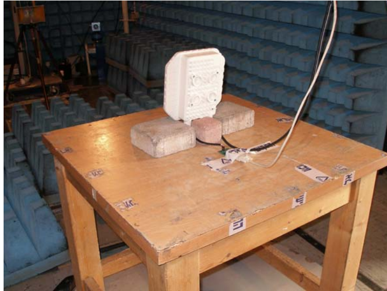
Photo #3. Test setup in anechoic chamber.
