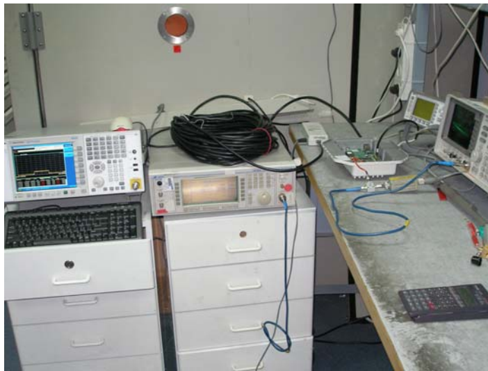
Photo #1. RF conducted emissions test setup.
