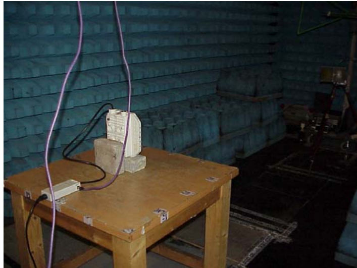
Photo #1. Spurious emissions investigation test in Anechoic chamber.
