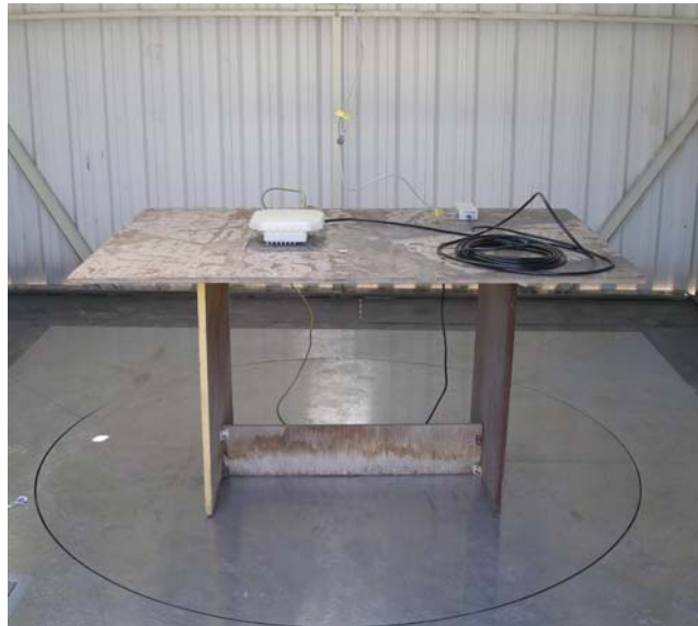
Photo #3. Radiated emissions test setup on OATS.
