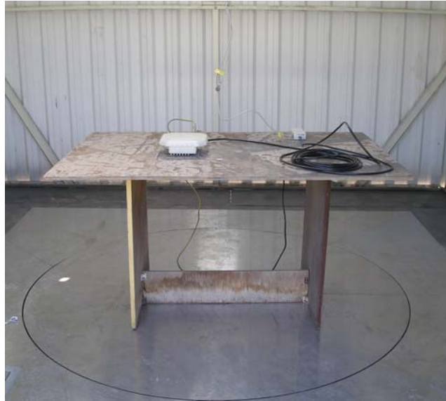
Photo #3. Radiated emissions test setup on OATS.
