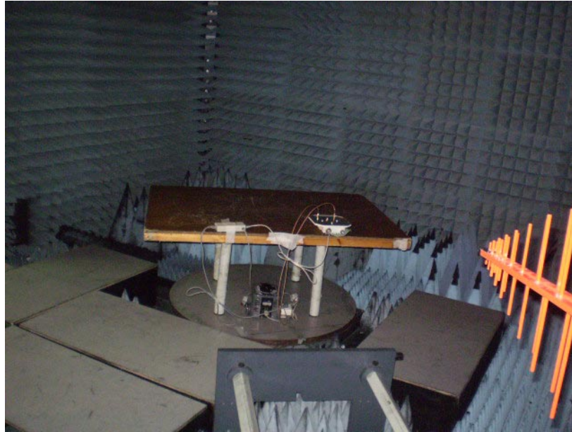
Photograph No.4 Spurious emissions measurement setup in the anechoic chamber in 30 -1000 MHz
