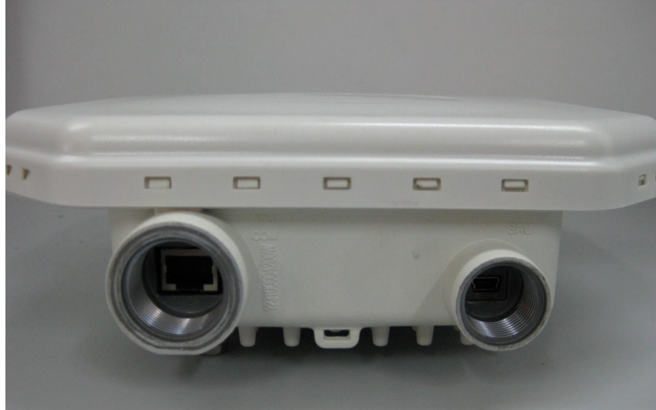
Photograph No.2 BreezeMAX Extreme 5GHz CPE connectors view
