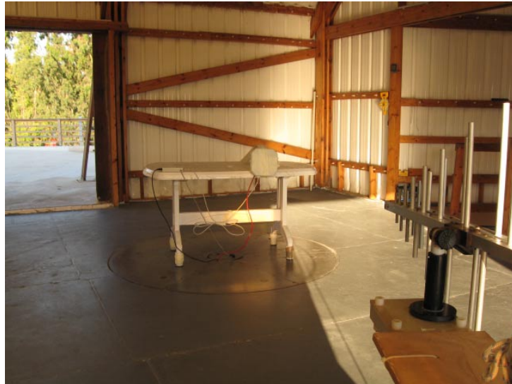
Photograph 8.2.5 Setup for radiated emission measurements at the OATS with log-periodic antenna
