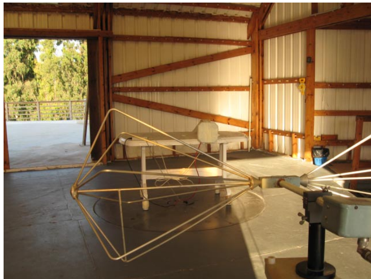
Photograph 8.2.4 Setup for radiated emission measurements at the OATS with biconical antenna
