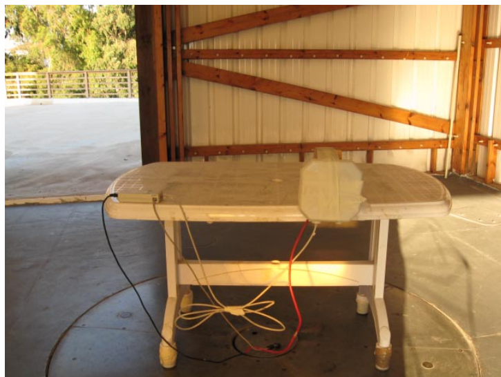
Photograph 8.2.6 Setup for radiated emission measurements, EUT cabling
