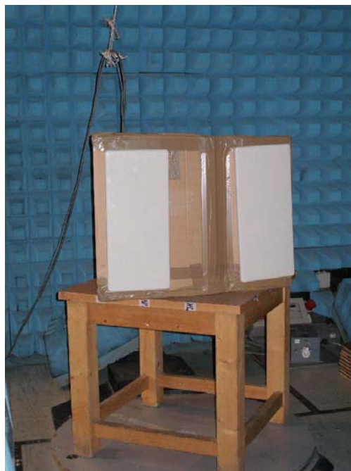
Photo #4. Test setup with external sector antennas.
