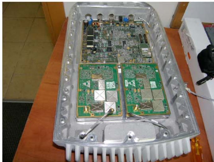
Photo #6. Outdoor unit. Internal view.
