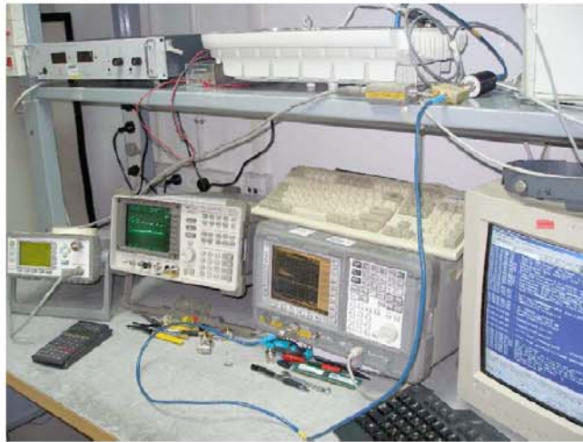
Photo #1. RF conducted emissions test setup.
