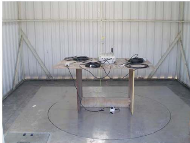
Photo #2. Radiated emissions test setup on OATS.
