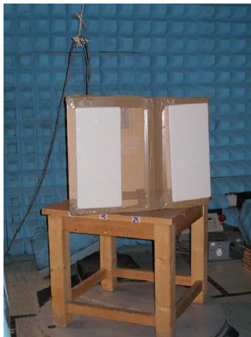
Photo #4. Test setup with external sector antennas.
