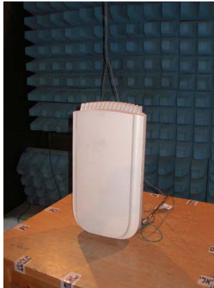
Photo #3. Radiated emissions test setup with internal antenna.
