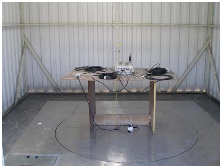
Photo #2. Radiated emissions test setup on OATS.
