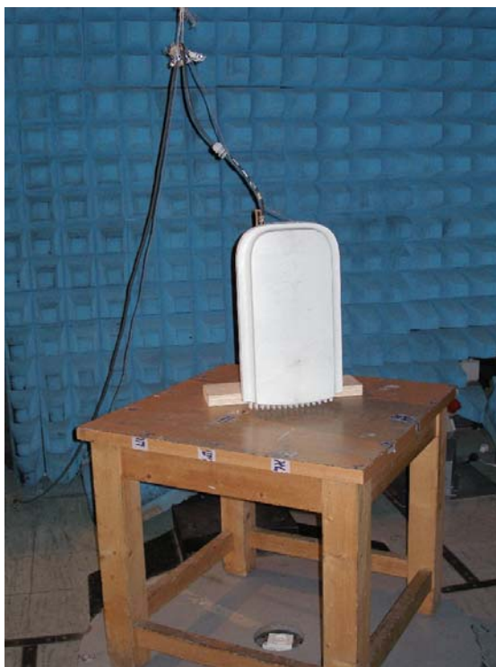
Photo 2. Test setup with internal antenna.
