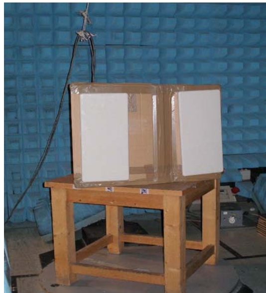
Photo 5. RE test setup with external sector antennas.
