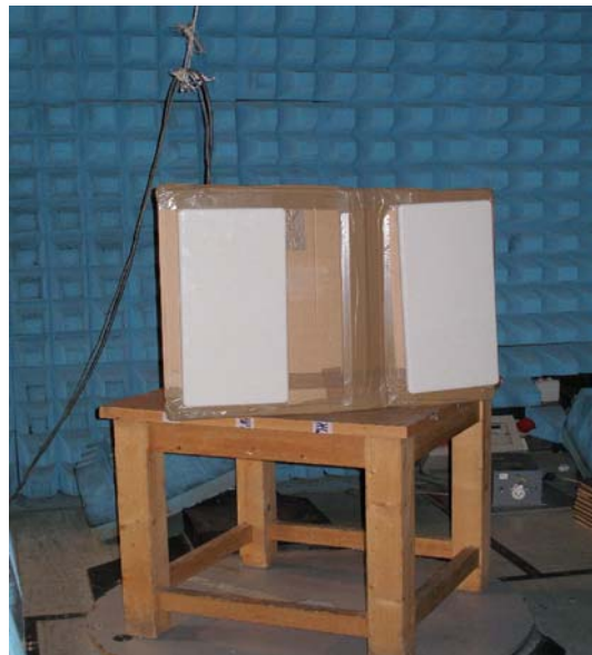
Photo 5. RE test setup with external sector antennas.
