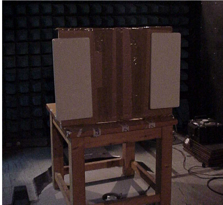
Photo 5. Investigation test setup with external sector antenna.
