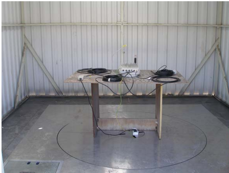
Photo 2. Test setup on OATS.
