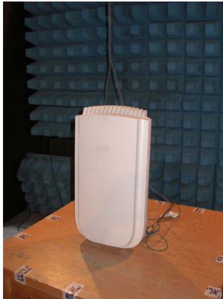
Photo 3. Investigation test setup with internal antenna.
