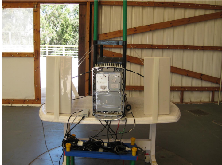
Photograph 8.2.3 Setup for radiated emission measurements, EUT cabling
