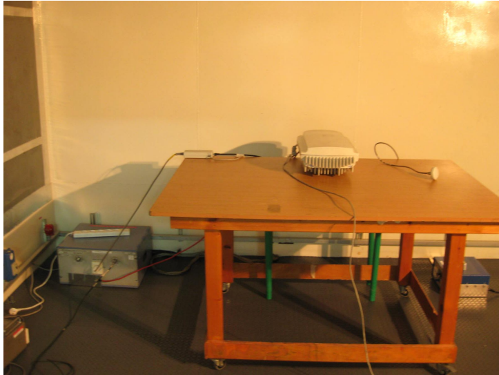
Photograph 8.1.2 Setup for conducted emission measurements
