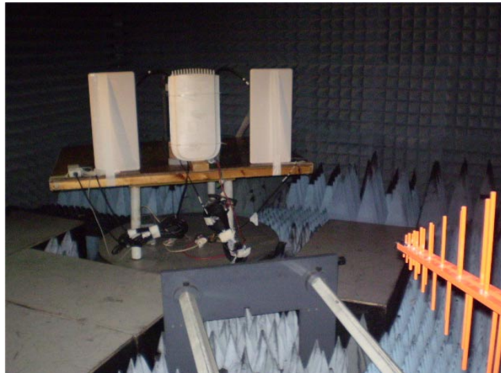
Photograph 8.2.1 Setup for radiated emission measurements in anechoic chamber
