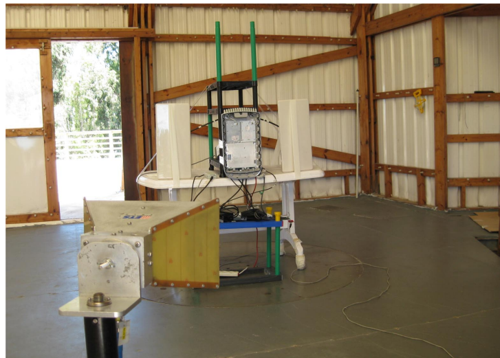
Photograph 8.2.2 Setup for radiated emission measurements at OATS, general view
