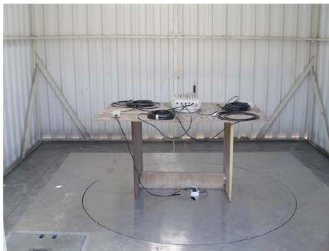
Photo 2. Test setup on OATS.
