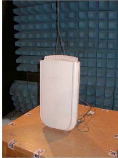
Photo 3. Investigation test setup with internal antenna.
