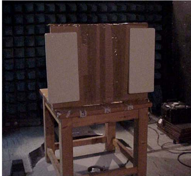
Photo 5. Investigation test setup with external sector antenna.
