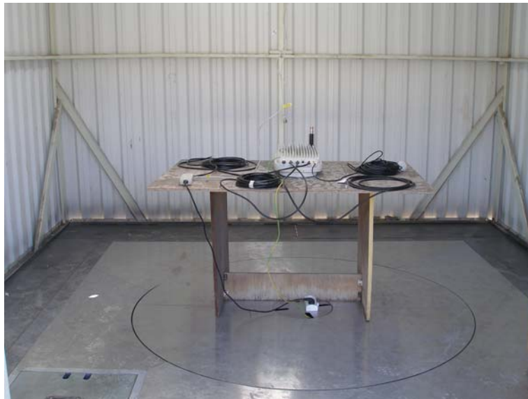
Photo 2. Test setup on OATS.
