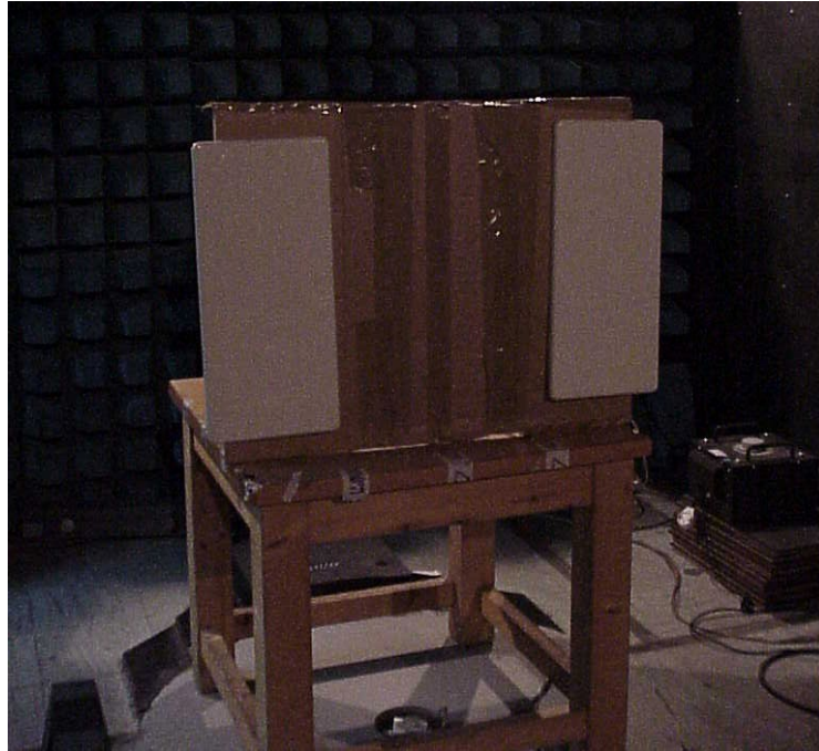
Photo 5. Investigation test setup with external sector antenna.
