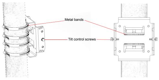
Figure 2-7: Installed Carriage with Metal Bands
