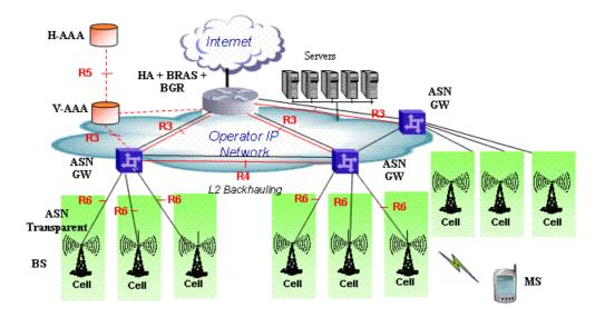
Figure 1-3: Centralized Network Reference Model
