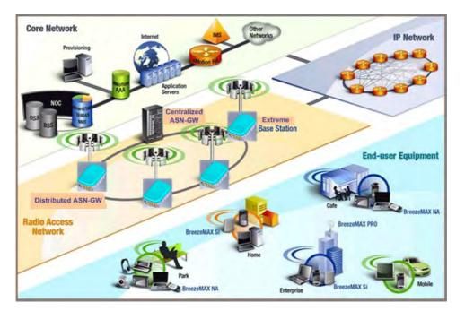
Figure 1-5: BreezeMAX Extreme System Architecture
