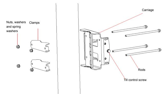
Figure 2-5: Assembling BTS Carriage and Clamps
