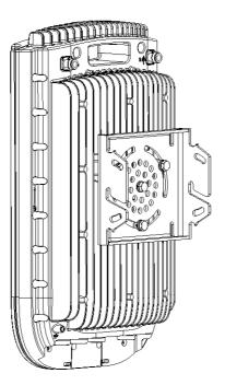
Figure 2-2: Tilt Bracket Installed on BTS
