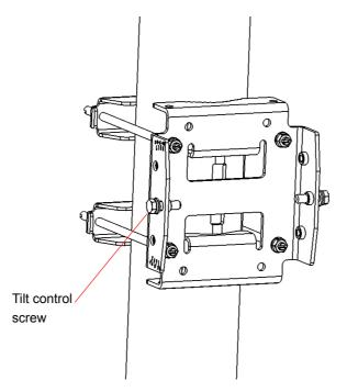
Figure 2-6: BTS Carriage and Clamps Installed
