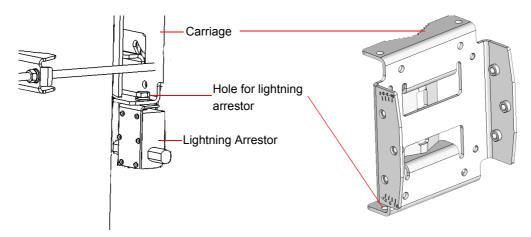
Figure 2-3: Installing the Lightning Arrestor on the Carriage
