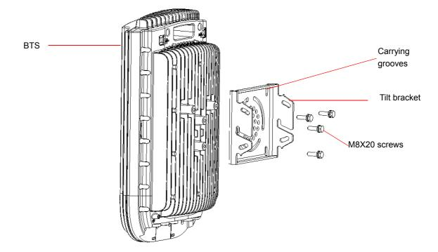
Figure 2-1: Assembling the Tilt Bracket on the BTS
