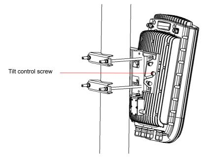
Figure 2-8: BTS Mounted on a 1.5"-4" Pole (with Clamps)
