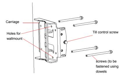
Figure 2-10: Mounting the Carriage on the Wall
