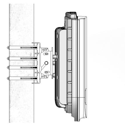
Figure 2-9: BTS Mounted on a Pole Larger than 4" (with Metal Bands)
