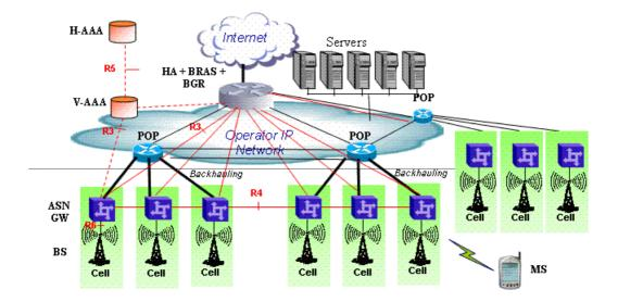
In the distributed approach, the BTS operates in ASN-GW mode, as shown in Figure 1-4.
