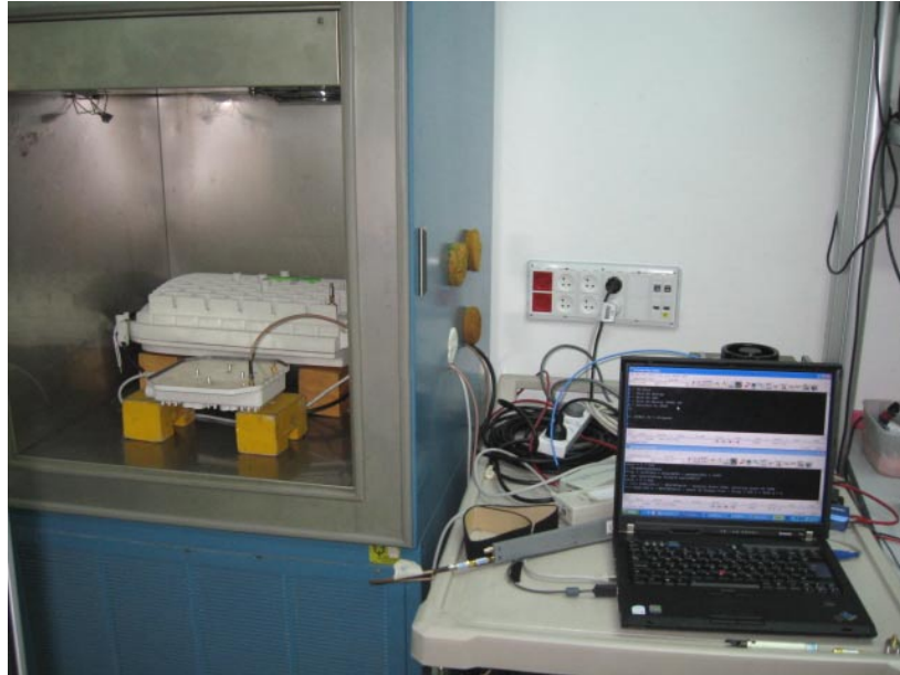
Photograph No.7 Frequency stability measurement setup
