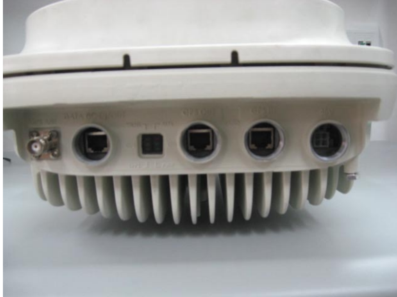
Photograph No.2 BreezeMAX Extreme 4.9GHz base station connectors view
