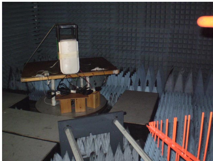
Photograph 8.2.1 Setup for radiated emission measurements in the full anechoic chamber
