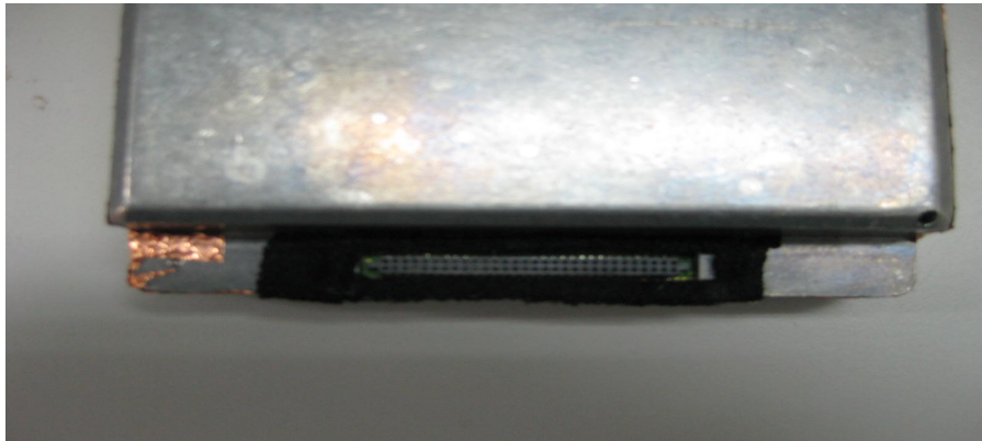
Photograph 6.7.2 RF head connector
