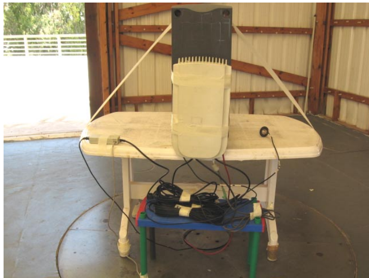
Photograph 8.2.2 Setup for radiated emission measurements at OATS, EUT cabling
