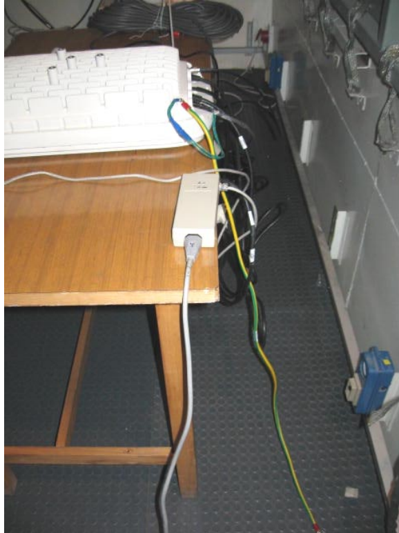
Photograph 8.1.2 Setup for conducted emission measurements
