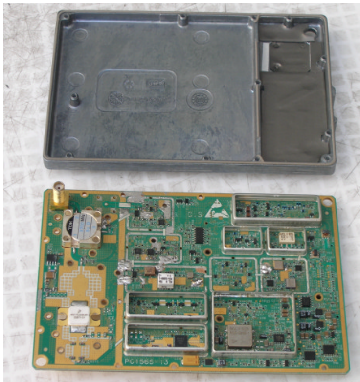
Photograph No.4 Radio module view without cover and shields
