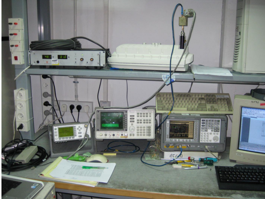
Photograph No.1 Peak output power, occupied bandwidth, emission mask measurement setup
