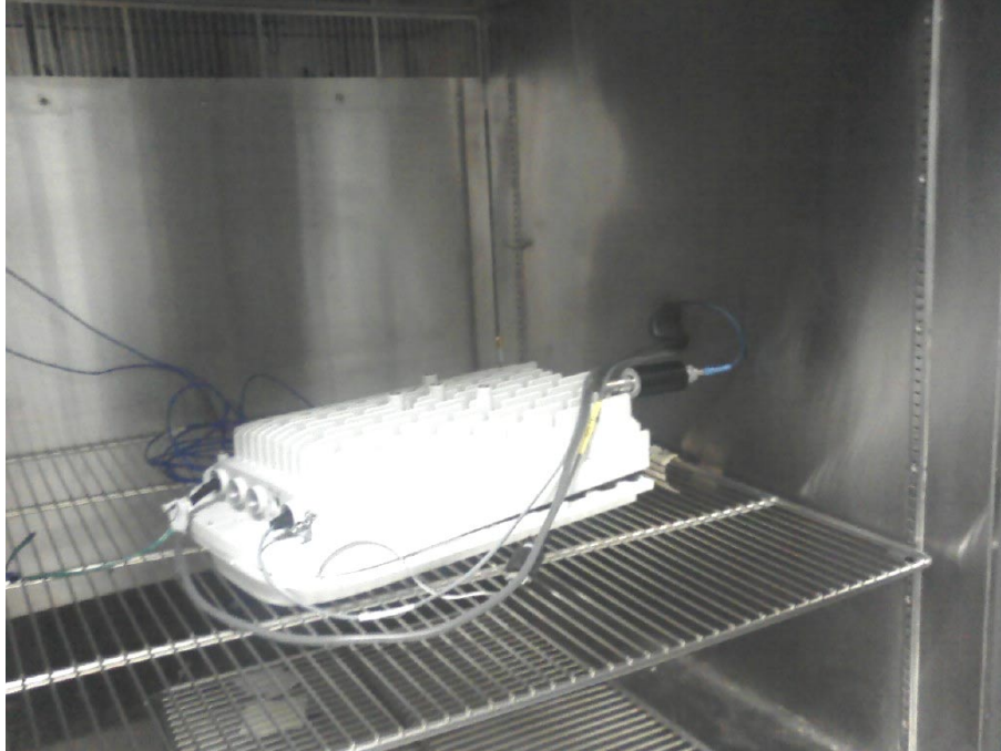
Photograph No.7 Frequency stability measurement setup
