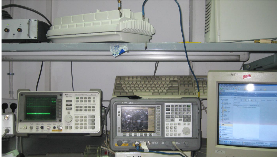
Photograph No.2 Conducted spurious emissions measurement setup
