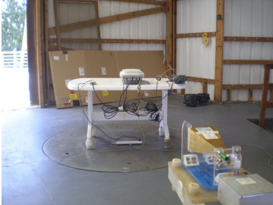
Photograph No.5 Radiated emissions measurement setup at the OATS above 1000 MHz
