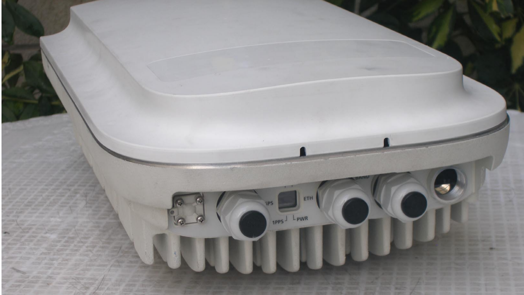
Photograph No.2 BreezeMAX Extreme 3.65 base station connectors view
