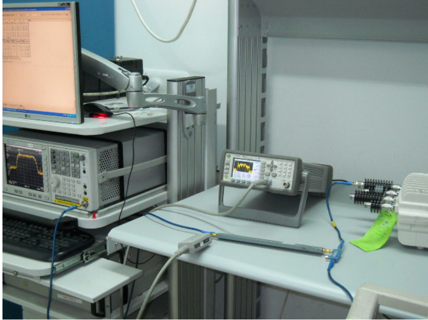
Photograph No.2 Peak power density, emission mask measurement setup
