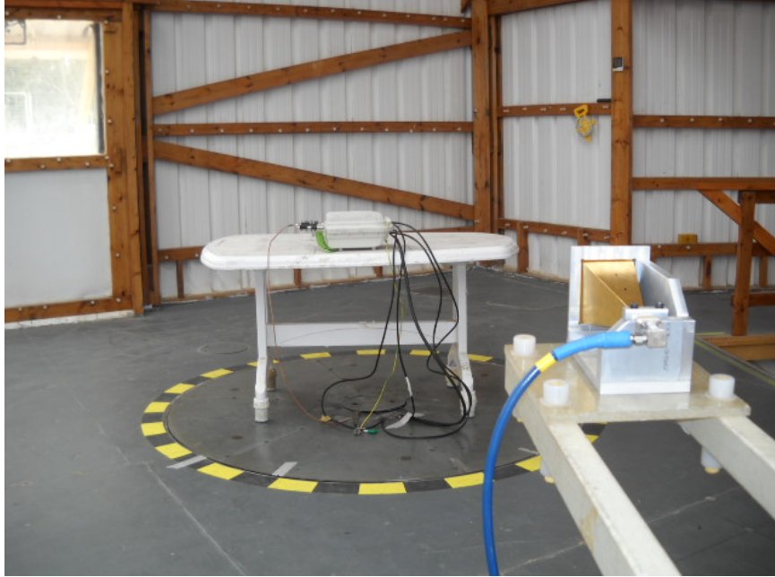
Photograph No.8 Radiated emissions measurement setup at the OATS in 26.5 – 37 GHz
