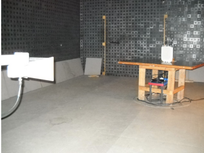
Photograph No.6 Radiated emissions measurement setup in the anechoic chamber in 1 - 18 GHz
