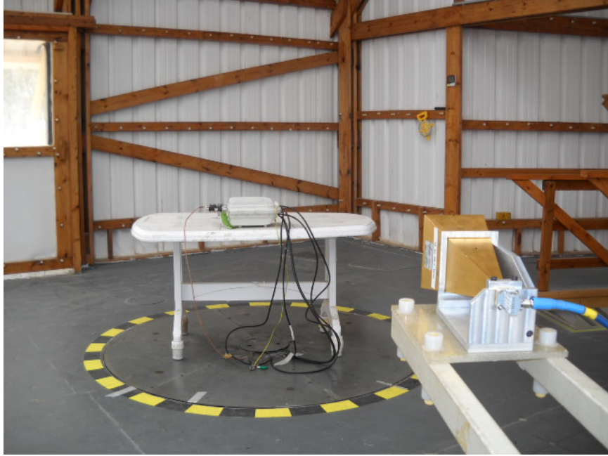
Photograph No.7 Radiated emissions measurement setup at the OATS in 18 – 26.5 GHz
