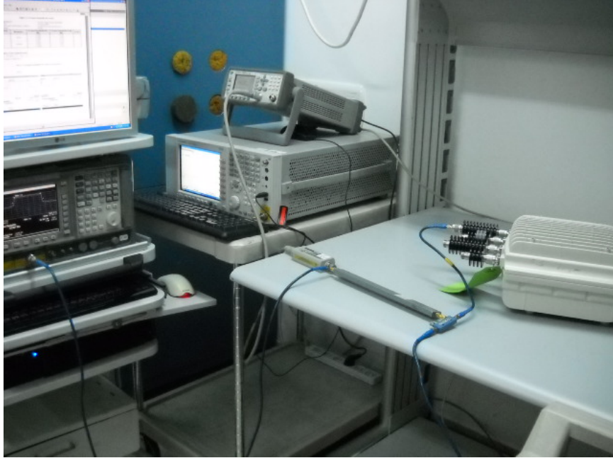
Photograph No.3 Occupied bandwidth, conducted spurious emissions measurement setup
