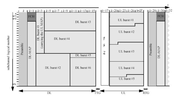
TTG is Transmission switching to Receive Gap in the BS and vice versa in the CPE. RTG is Receive switching to Transmit Gap in the BS and vice versa in the CPE.
