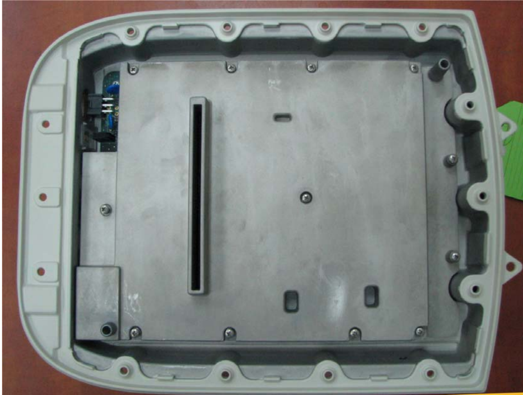
Photograph No.6 BreezeCOMPACT base station digital part internal view
