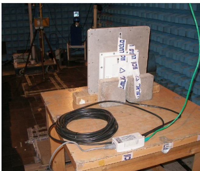
Photo 3. Radiated emissions test setup with internal antenna.
