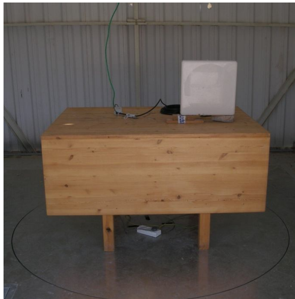
Photo 2. Radiated emissions test setup on OATS.
