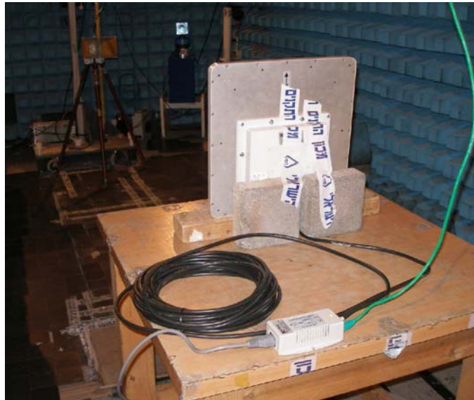
Photo 3. Radiated emissions test setup with internal antenna.
