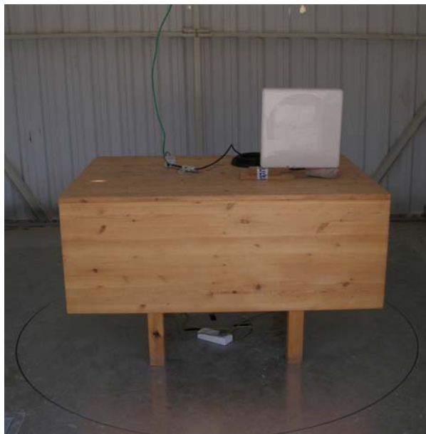
Photo 2. Radiated emissions test setup on OATS.
