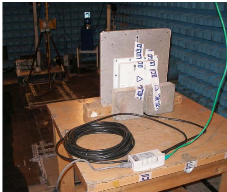
Photo #2. Radiated emissions test setup in anechoic chamber.
